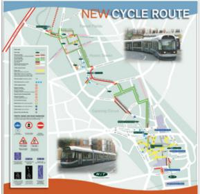
This cycling map of the Nottingham tram system shows signalized crossings, alternate routes, bicycle parking locations, and the meaning of pavement markings.
