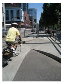
At this sidewalk detour in Portland, pavement markings and railings differentiate between cyclist and pedestrian zones.
