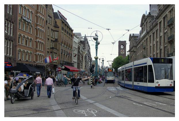
This photo from Amsterdam illustrates many of the international best practices identified above: spatial separation of the cycle track from tram tracks, center-running tracks and platforms, separation of bicyclists and pedestrians, clear pavement markings directing cyclists, and near-perpendicular track crossing angles. Source: <u>http://www.flickr.com/photos/anw-fr/2744645044/</u> (used with permission)
