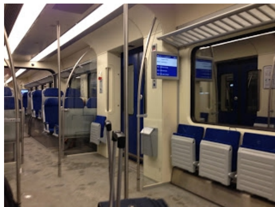
Dutch train, with a useful mix of fixed and flexible seating
