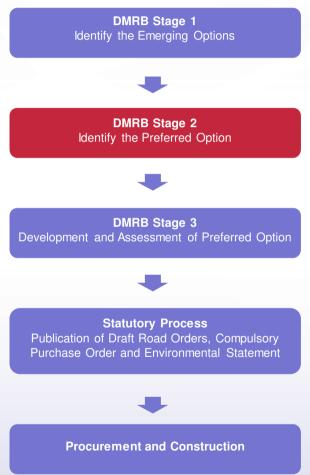
A rigorous assessment process is required to determine the preferred option for a trunk road improvement scheme.
