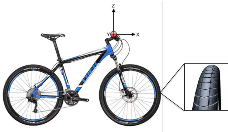
Figure 1: Mounting position for accelerometers and tyre tread pattern.
