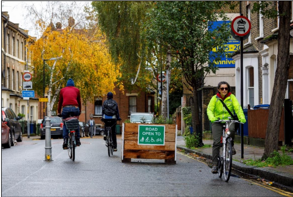
Figure 2:3: Modal filter bollard and signage in Walworth, London (credit: Sustrans)
