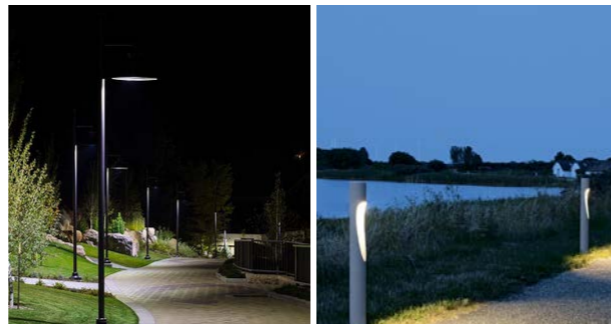
Alternative luminaires, with less direct views of the sources, would reduce glare and focus light onto pathways
