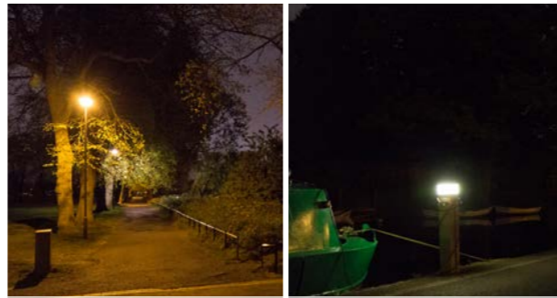
Visible existing light sources alongside Harrison Park introduce discomfort glare and reduced visibility for pedestrians.
