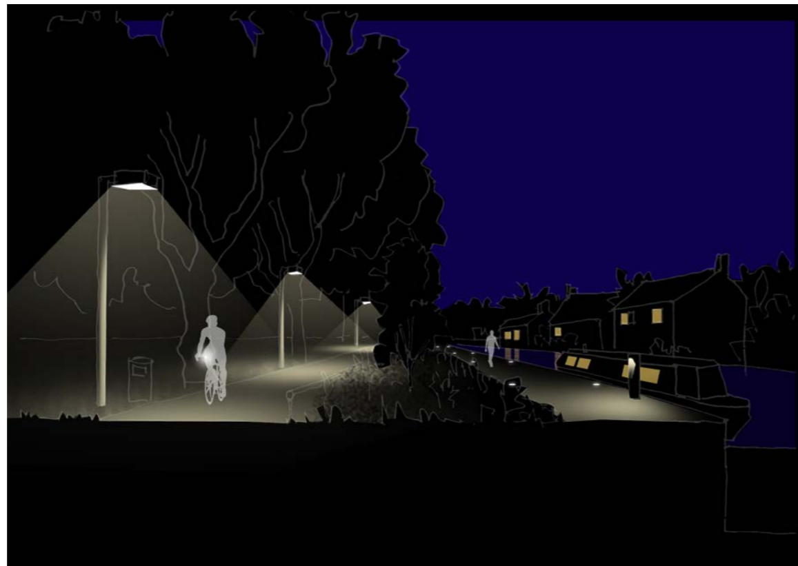
Alternative luminaires, with less direct views of the sources, would reduce glare and focus light onto pathways
