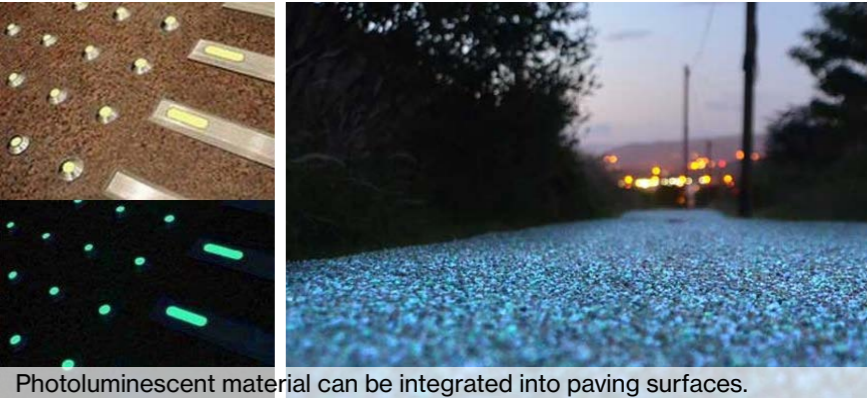
Photoluminescent material can be integrated into paving surfaces.
