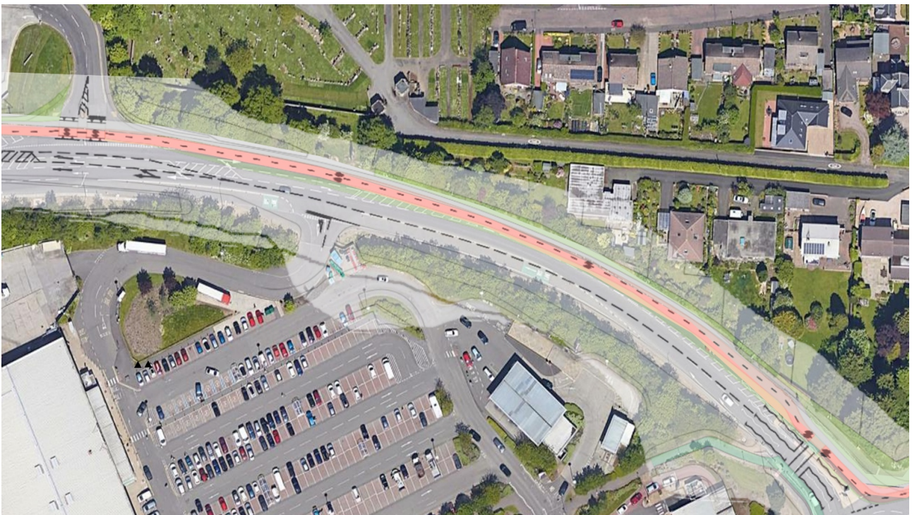
Plan of Ferry Muir Road with segregated cycle track on north side
