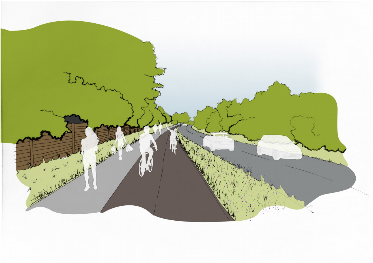
Plan showing reallocated road space on northern bridge of Echline Junction for walking, wheeling and cycling only. Motor vehicles would use southern bridge
